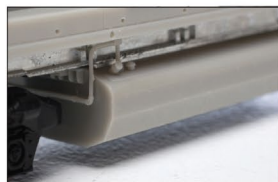
NS specific crash-worthy fuel tank per prototype
