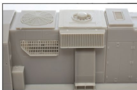
Rebuilt inertial/clean room
