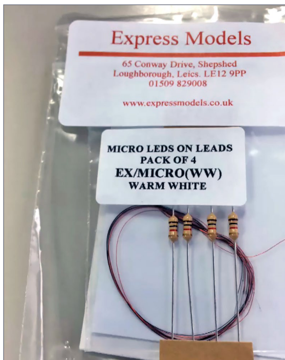
5. Express Models supplied micro LEDs and resistors I used.
