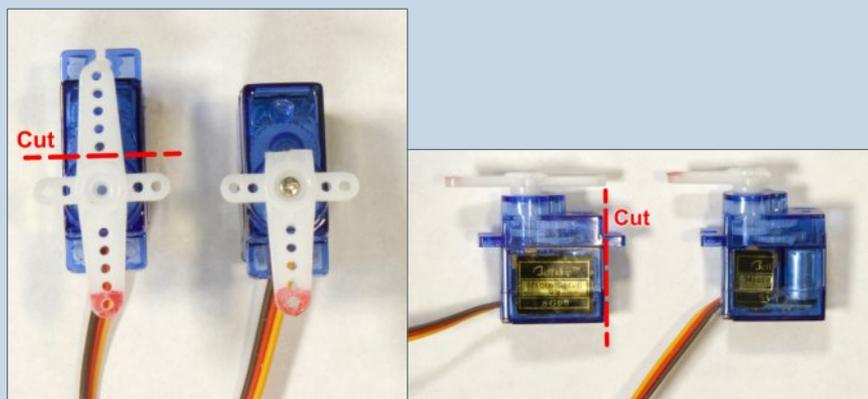
8, 9. Once I've determined 90 degrees on a new servo, I add the horn and use flush cutters to clip the top arm off (left image). Then I use a razor saw (right image) to cut off the servo body tab on the side opposite the wires.
