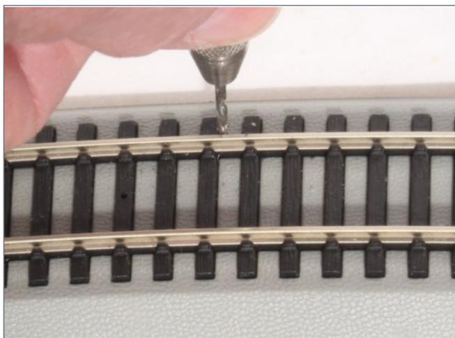
13. Drill a 1/16-inch hole next to the base of the rail.
