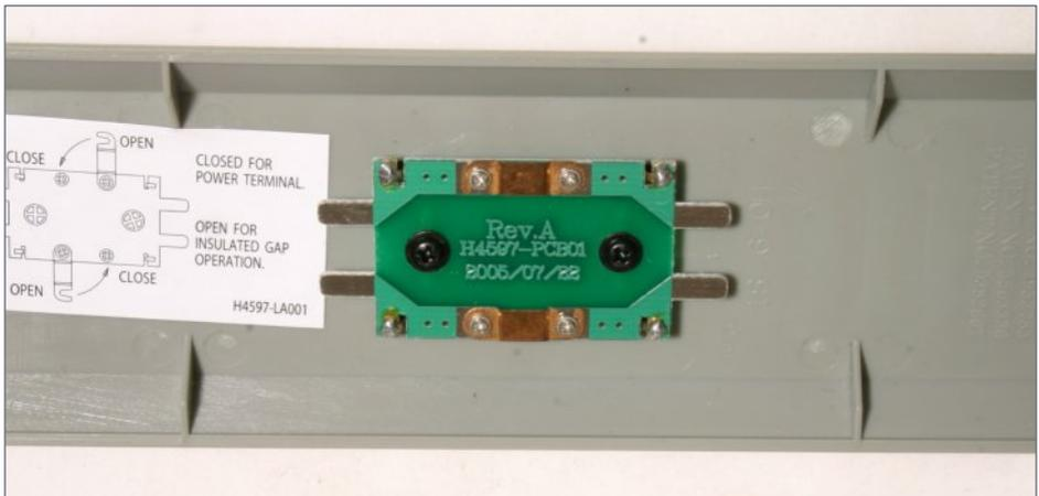
**11.** The E-Z Track 9" terminal rerailer can be used either as power-connector or to provide an electrical insulation gap.
