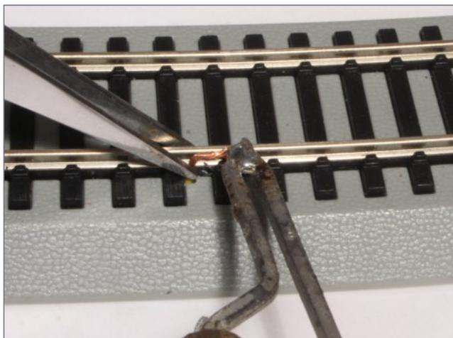
16. Touch the tip of the soldering gun to the outside edge of the wire while you also position the solder against the bare wire. Try to keep the tip away from the solder. You want the rail to get hot enough to melt the solder. Once the solder melts, it
