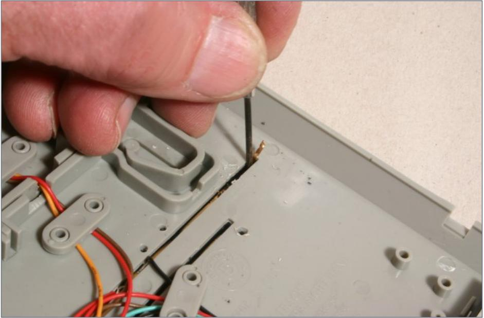
22. Pry the copper strips loose from the bottom of the turnouts, and remove them. Finally, connect the inner rails with wires to route power around the frogs, as shown for modifying the single turnouts.
