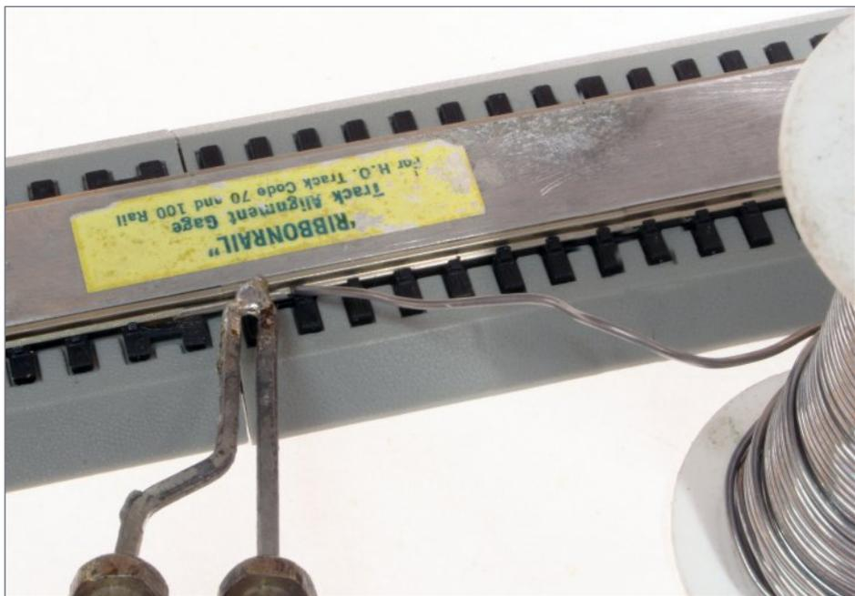
5. I used a 100-watt soldering gun with 50/50 rosin-core solder. I touched the tip of the gun to the rail joiner, positioned the solder against the top corner, and removed the gun the moment flow occurred. It pays to practice this technique on old track sections.
