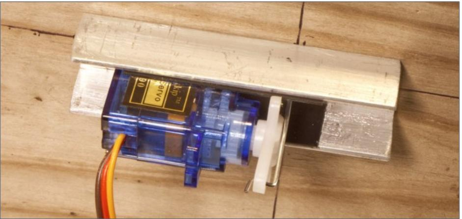
14. Next I thread the wire up through the hole in the aluminum channel, and thread the wire topside through the hole in the throw bar. Then I press the servo firmly into the channel, aligning the wire so it's nicely vertical underneath the throw bar. With this, we're ready to begin configuring the final servo throw!
