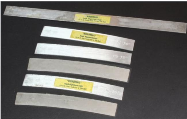
3. I used Ribbonrail (Baumgarten) rail gauges to hold the rails at the track joint during soldering. These six gauges match the available radii from E-Z Track: 22, 26, 28, 32 and 35
