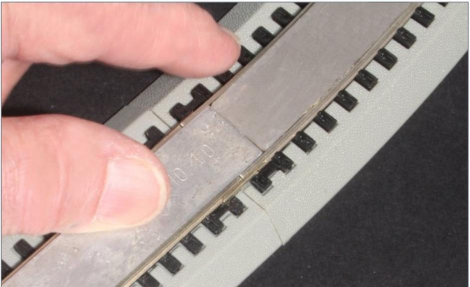
4. To be sure there are no kinks where a curve joins a straight, I slide a straight gauge about 1/2-inch into the curve and hold the curve with the proper-size curve gauge.
