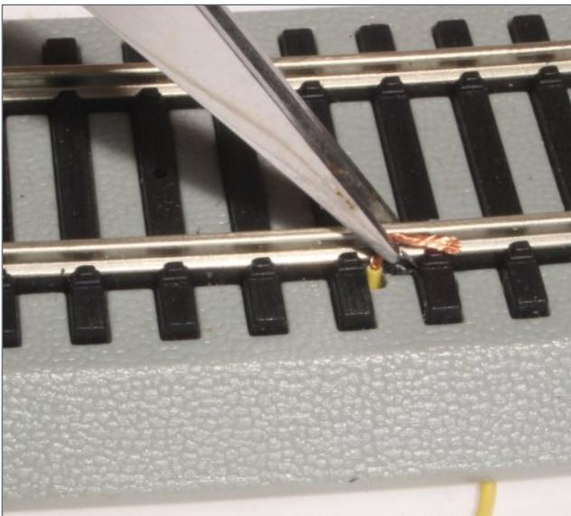
15. Use tweezers to hold the end of the wire's insulation against the web on the outside of the rail.
