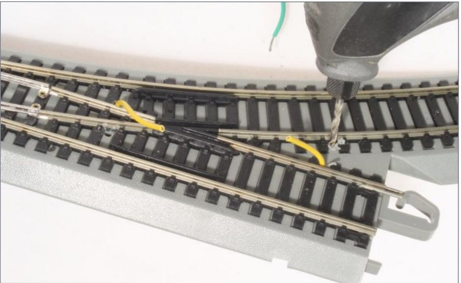
18. Drill four 1/16-inch holes to the outside of both outer rails so these yellow and green "jumper" wires can be installed.
