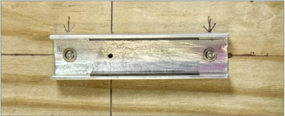
12. Once I had the starter holes for the mounting screws drilled, I mounted the aluminum channel on the underside of the roadbed with the mounting screws shown in [10]. Note how the half-inch hole crosshairs from [6] make aligning the aluminum channel easy – just make sure the throwbar wire hole is in the center of the crosshairs.
