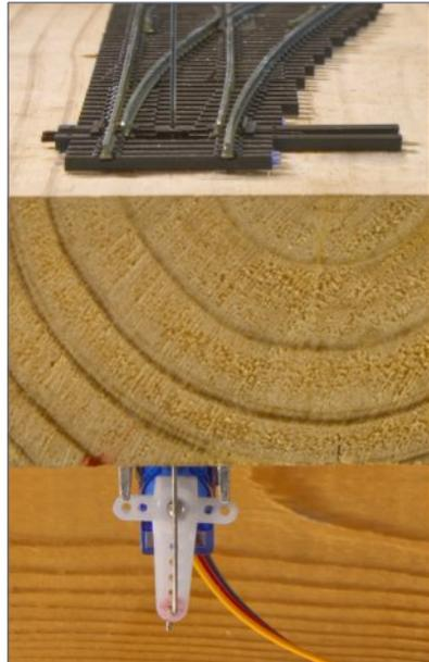
15, 16. Once the servo has been mounted in a centered position, this is how it should look. The turnout points should be centered between the two stock rails, and the servo horn should be pointing down in a vertical position. Now we're ready to set the turnout throw using the calibration sketch.
