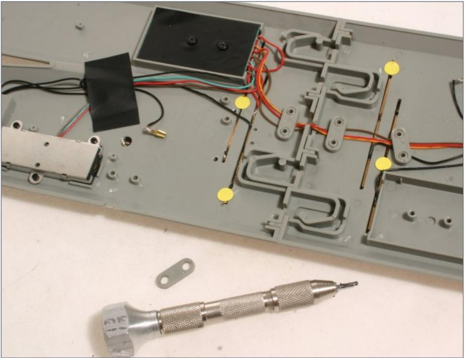
21. E-Z Track crossovers are also wired so both routes are powered. To modify the crossover so power is directed only to the selected route, cut the four thin copper strips on the bottom of the turnout. Use a 1/16" bit to drill through the strips at the points indicated by the yellow dots. Remove the small dumbbell-shaped tabs covering the copper contacts.
