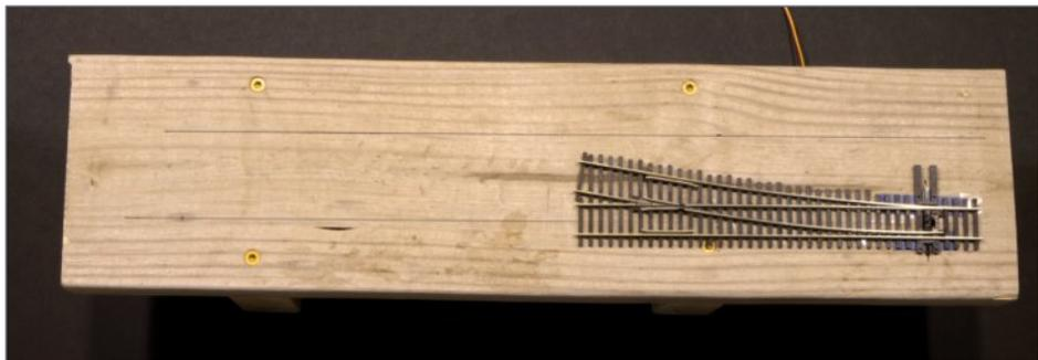
5. Overhead view of my turnout test fixture. This view shows the #6 Peco Unifrog turnout I later mounted on the board after drilling the half-inch hole [6] on one end.
