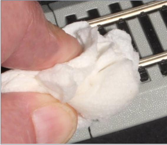
**6. Allow the solder to cool. Scrub the joint with a damp paper towel to remove any soldering rosin.**
