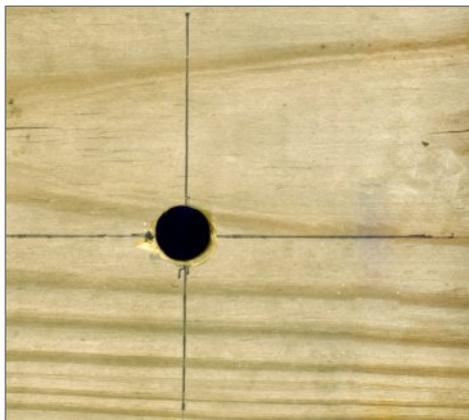
6. I drilled a half-inch hole two inches from one end centered on the front track centerline. On the bottom, I added hole centerline crosshairs to make aligning the servo mounting channel easier. considerable space when that's needed.
