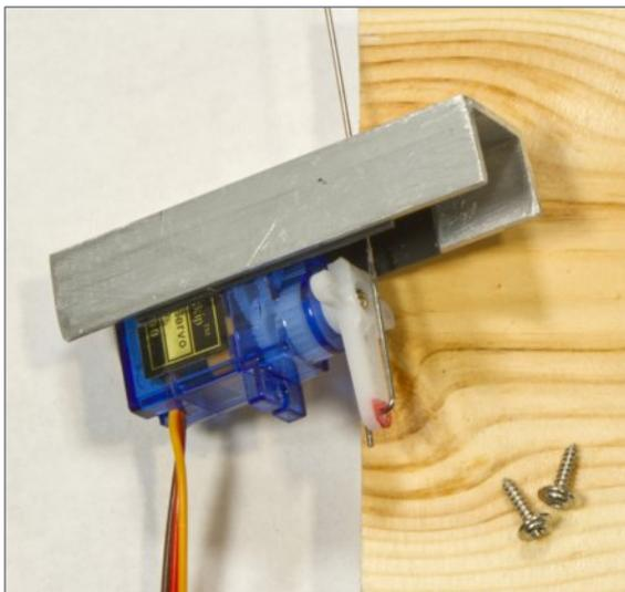
10. I use a length of half-inch aluminum channel to mount the servo underneath the turnout. For mounting screws, I just use the large screws shown here that come with the servo.
