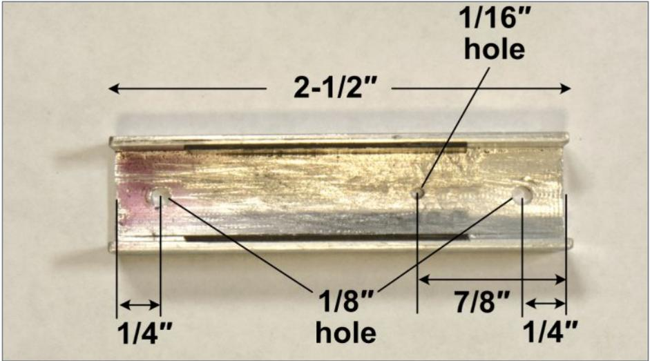
11. Servo mounting bracket dimensions as seen in [10]. Note the 0.020" black styrene I super-glued along the sides – I needed to add that to get a snug-enough fit so the servo would not move around.
